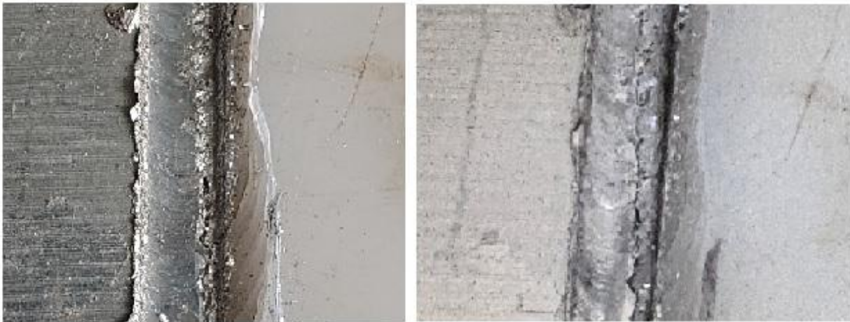
Fig.5: Macrostructure of Disimilar FSW joint Aluminium AA 8090 and PP
