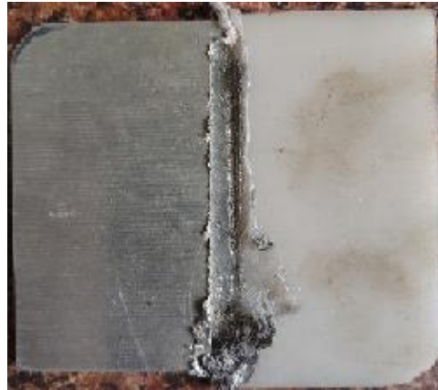
Fig.3: CFR Polymer and AA 8090 Dissimilar Feasible Joint Formation
