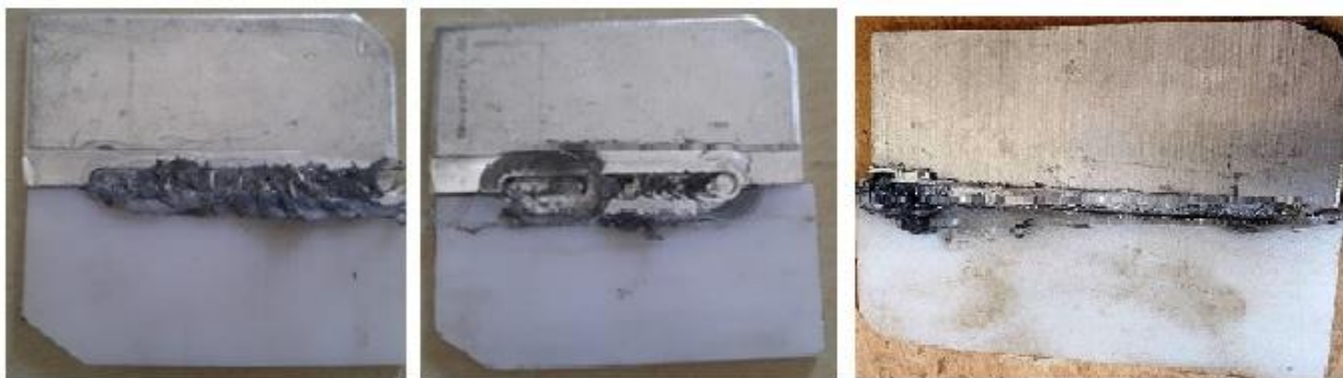
Fig.2: CFR Polymer and AA 8090 Dissimilar Joint Formation
