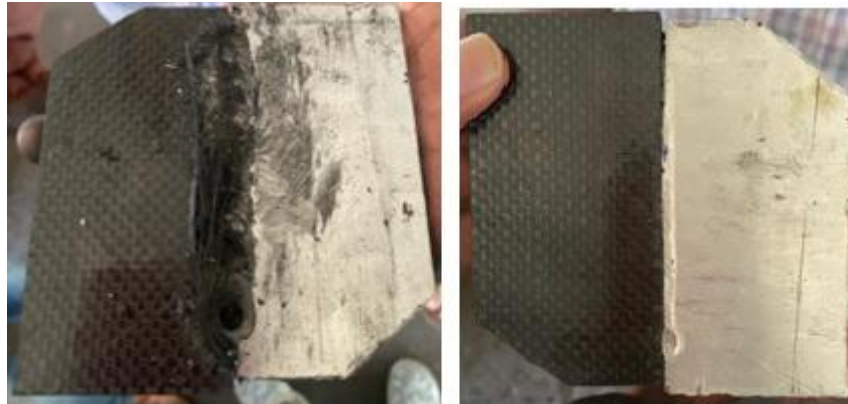
Fig1: CFR Polymer and AA 8090 Dissimilar Joint Formation
