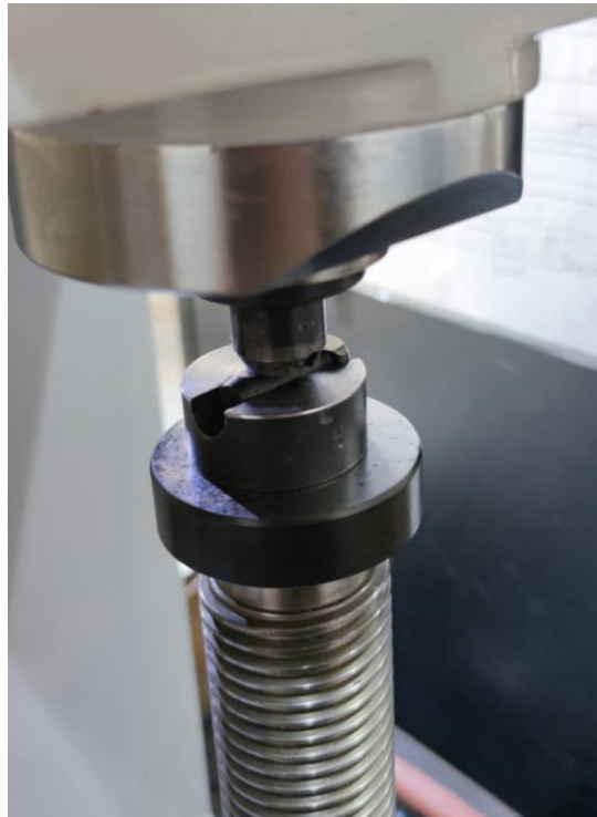
Fig 10. Hardness Testing Process of Nissan Junior Blind Rivet After Tempering Heat Treatment
