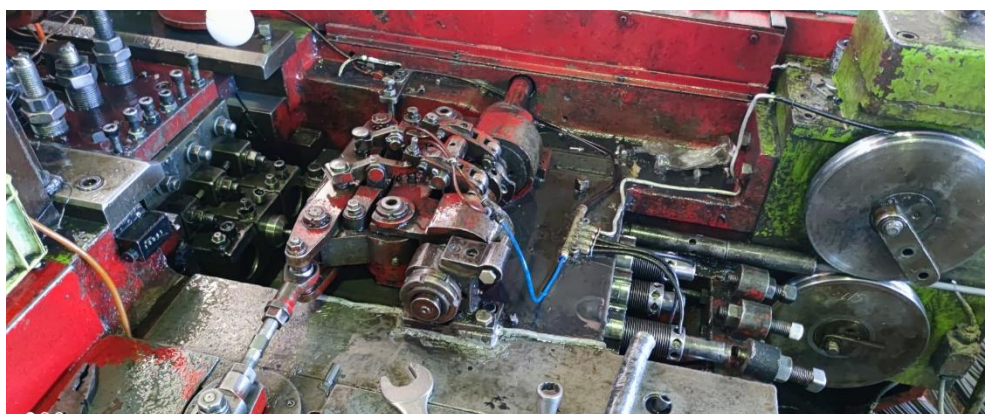
Fig4. A view of the P8 single-stroke four-die machine, which was initially used for producing the Nissan Junior blind rivet
