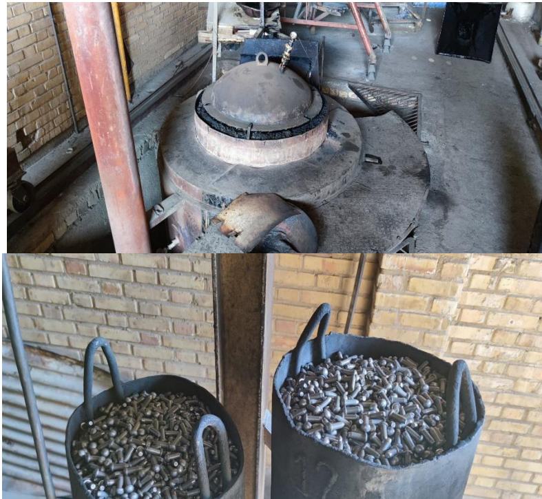
Fig9. The heat treatment furnace built at Koobesh Kavir Semnan Factory, along with the tubes prepared for charging the furnace
