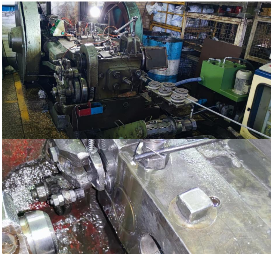
Fig6. P10-1 Machine Used for the Current Production of Nissan Junior Blind Rivet
